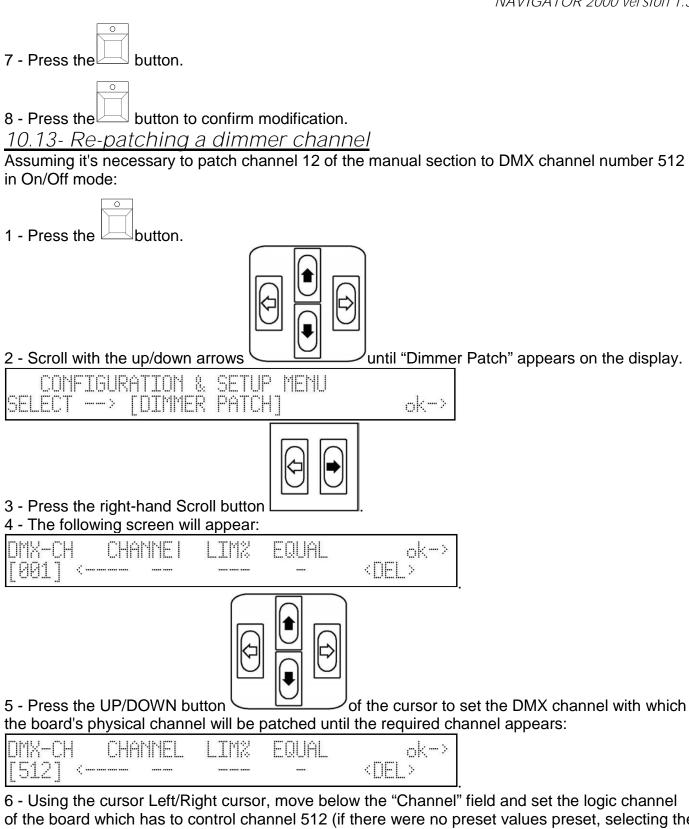
of the board which has to control channel 512 (if there were no preset values preset, selecting the logic channel automatically creates the LIM% and EQUAL "fields"):
